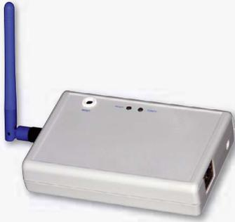
**Wireless LAN Access Point with ETHERNET interface for operation with a FVS-Safe server in conjunction with the FVS-Professional Wireless Visualisation and Control Software.**
